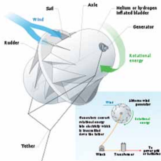
Fig 4. Airborne wind generator of Savonius style (source Wikipedia)
