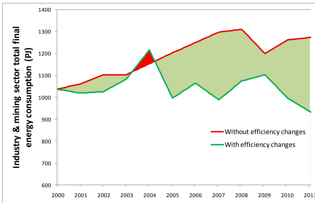
Figure 11 Comparison of actual observed trends in energy consumption of the industry & mining sector (green trace) versus trends that would have occurred with no efficiency change (red trace).
